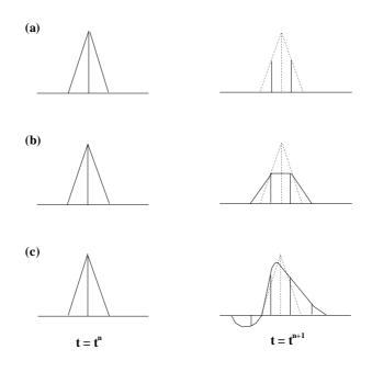
Figure 1: Numerical problems caused by advection (a) peak clipping (b) numerical diffusion (c) spurious oscillation and phase error, [28]
