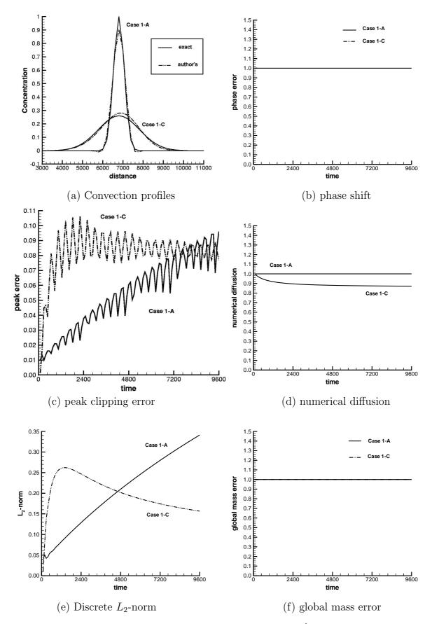
Figure 4: Comparison of Cases 1-A and 1-C with  $\Delta t < \frac{\Delta x}{u}$  after 100 time steps
