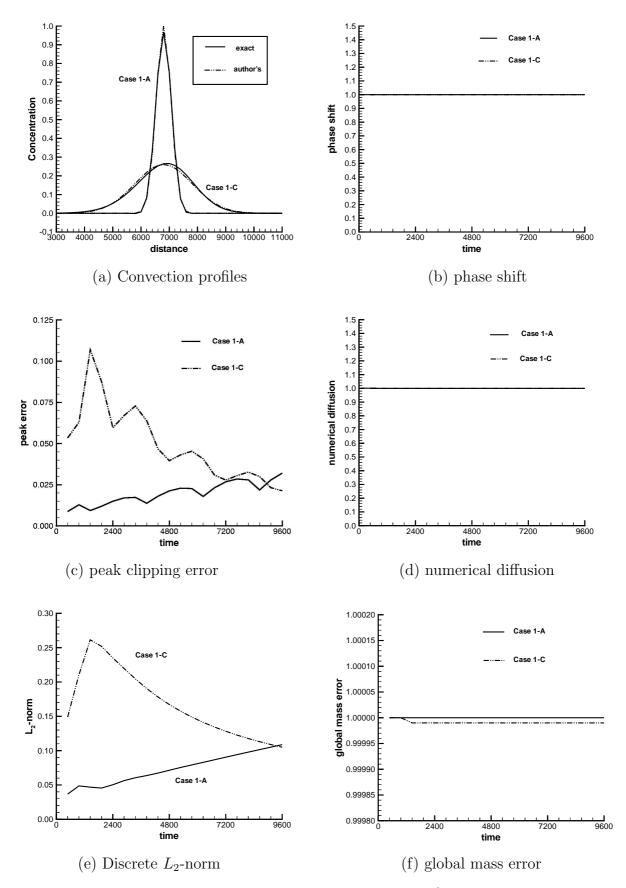
Figure 5: Comparison of Cases 1-A and 1-C with  $\Delta t > \frac{\Delta x}{u}$  after 20 time steps
